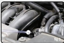
**NOTE:** Connect the applicator tip to a strong manifold vacuum source as close to the throttle plate as possible to distribute cleaning solution to all cylinders (fig 3). The selected vacuum hose originates from central and just behind the throttle plate. Always select a location like this. **NEVER** use a vacuum port that originates from an individual intake runner.
